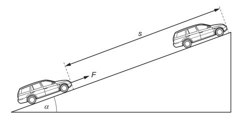
What is the ratio gravitational potential energy gained by car ? work done by force F
