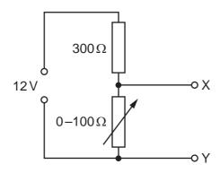
Which range of voltages can be obtained between X and Y?
