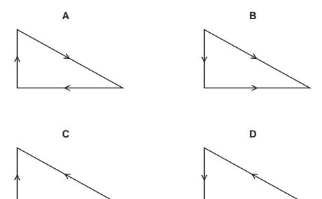
14 Two rigid steel beams XY and YZ are fixed at their lower ends and are hinged at Y. Each beam is inclined at  $50^{\circ}$  to the horizontal, as shown. A weight of  $4.0 \times 10^4$  N hangs from Y. The structure is in equilibrium.
