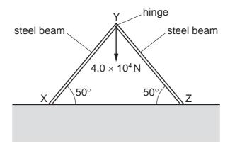
What is the force exerted by each beam on the hinge at Y?
