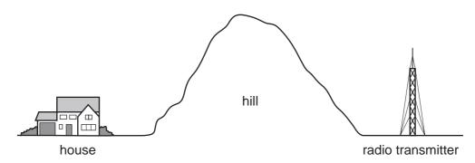
The radio transmitter cannot be seen from the house, but radio waves from the transmitter are received at the house.
