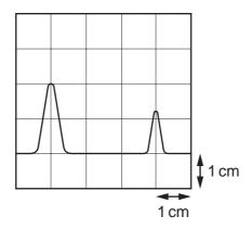
The pulse takes 6.3 µs to travel from the transmitter to the reflector.
