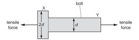
The bolt has a circular cross-section. At end X the diameter is 2d. At end Y the diameter is d.
