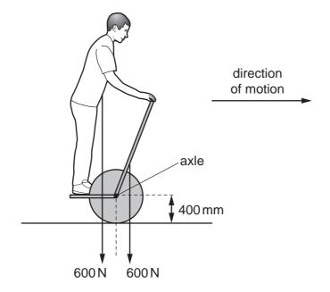
The vehicle has two wheels on one axle. The passenger stands on a platform between the wheels.
