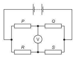
The voltmeter reading is zero.
