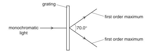
The spacing of the slits in the grating is  $1.00 \times 10^{-6}$  m. The angle between the first order diffraction maxima is 70.0°.
