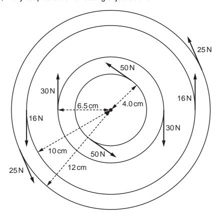
What is the resultant torque acting on the rotating object?
