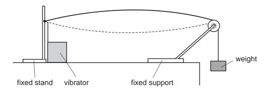
A vibrator is attached to the wire near the clamped end. A stationary wave with one loop is produced. The frequency of the vibrator is f.
