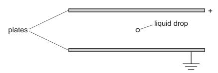
A small charged liquid drop, midway between the plates, is held in equilibrium by the combination of its weight and the electric force acting on it.
