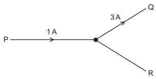
How much charge passes a given point in wire R in a time of 5s?
