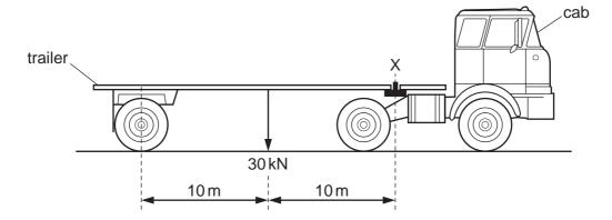
What is the upward force exerted at X by the cab on the trailer?
