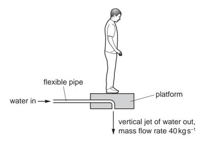
The resultant vertical force on the platform is zero. The combined mass of the man and platform is 96 kg. The mass of water that is discharged vertically downwards from the platform each second is 40 kg.
