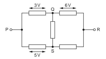
The potential difference (p.d.) between P and Q is 3V.
