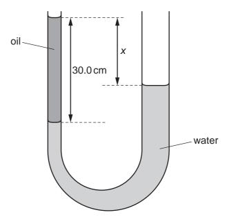
The column of oil on top of the water in the left-hand arm is of length 30.0 cm.
