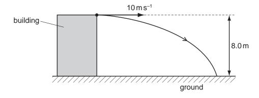
How long does it take the stone to reach the ground? (Air resistance can be neglected.)
