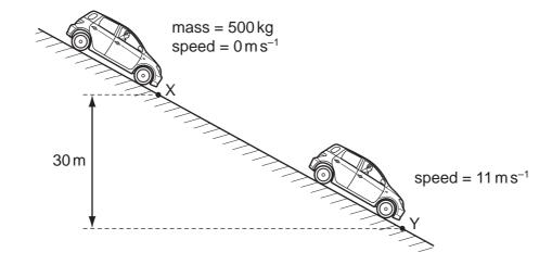
What is the energy dissipated by frictional forces when the car moves from X to Y?
