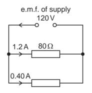
What is the internal resistance of the power supply?
