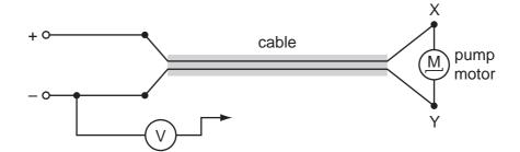
The motor does not work so, to find the fault, the negative terminal of a voltmeter is connected to the negative terminal of the power supply and its other end is connected in turn to terminals X and Y at the motor.
