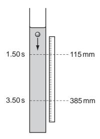
There are two marks on the tube. The top mark is positioned at 115  $\pm$  1 mm on the adjacent rule and the lower mark at 385  $\pm$  1 mm. The ball passes the top mark at 1.50  $\pm$  0.02 s and passes the lower mark at 3.50  $\pm$  0.02 s.
