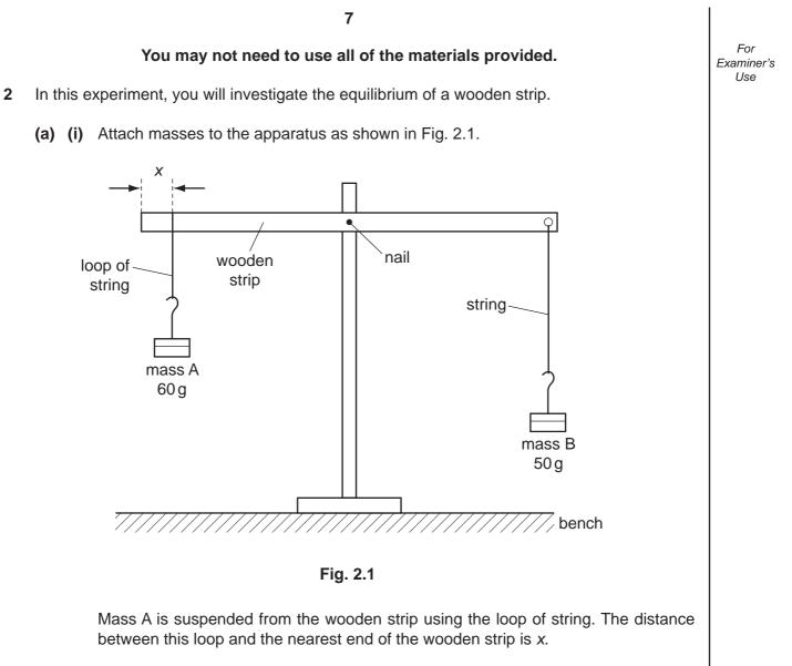
(ii) Change *x* until the wooden strip is balanced and approximately parallel to the bench. Measure and record *x*.
