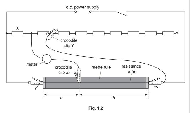
Only the first resistor in the chain is included in the circuit. This has resistance R of  $1000 \Omega$ .
