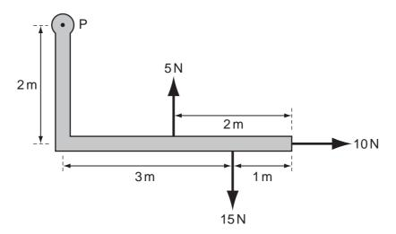
Three forces act on the lever arm, as shown in the diagram.
