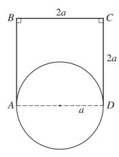
Three identical uniform rods, AB, BC and CD, each of mass M and length 2a, are rigidly joined to form three sides of a square. A uniform circular disc, of mass  $\frac{2}{3}M$  and radius a, has the opposite ends of one of its diameters attached to A and D respectively. The disc and the rods all lie in the same plane (see diagram). Find the moment of inertia of the system about the axis AD.
