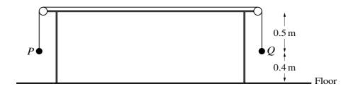
Particles P and Q, of masses 7 kg and 3 kg respectively, are attached to the two ends of a light inextensible string. The string passes over two small smooth pulleys attached to the two ends of a horizontal table. The two particles hang vertically below the two pulleys. The two particles are both initially at rest, 0.5 m below the level of the table, and 0.4 m above the horizontal floor (see diagram).
