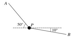
The diagram shows a small object P of mass 20 kg held in equilibrium by light ropes attached to fixed points A and B. The rope PA is inclined at an angle of 50° above the horizontal, the rope PB is inclined at an angle of 10° below the horizontal, and both ropes are in the same vertical plane. Find the tension in the rope PA and the tension in the rope PB. [5]
