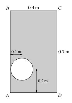
A uniform object is made by drilling a cylindrical hole through a rectangular block. The axis of the cylindrical hole is perpendicular to the cross-section *ABCD* through the centre of mass of the object. AB = CD = 0.7 m, BC = AD = 0.4 m, and the centre of the hole is 0.1 m from AB and 0.2 m from AD (see diagram). The hole has a cross-section of area  $0.03 \text{ m}^2$ .
