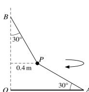
*OA* is a rod which rotates in a horizontal circle about a vertical axis through *O*. A particle *P* of mass 0.2 kg is attached to the mid-point of a light inextensible string. One end of the string is attached to the rod at *A* and the other end of the string is attached to a point *B* on the axis. It is given that OA = OB, angle OAP = angle  $OBP = 30^{\circ}$ , and *P* is 0.4 m from the axis. The rod and the particle rotate together about the axis with *P* in the plane OAB (see diagram).
