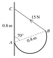
A uniform wire has the shape of a semicircular arc, with diameter AB of length 0.8 m. The wire is attached to a vertical wall by a smooth hinge at A. The wire is held in equilibrium with AB inclined at 70° to the upward vertical by a light string attached to B. The other end of the string is attached to the point C on the wall 0.8 m vertically above A. The tension in the string is 15 N (see diagram).
