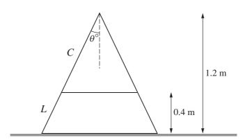
A uniform solid cone of height 1.2 m and semi-vertical angle  $\theta^{\circ}$  is divided into two parts by a cut parallel to and 0.4 m from the circular base. The upper conical part, C, has weight 16 N, and the lower part, L, has weight 38 N. The two parts of the solid rest in equilibrium with the larger plane face of L on a horizontal surface and the smaller plane face of L covered by the base of C (see diagram).
