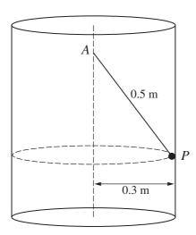
A smooth hollow cylinder of internal radius  $0.3 \,\mathrm{m}$  is fixed with its axis vertical. One end of a light inextensible string of length  $0.5 \,\mathrm{m}$  is fixed to a point A on the axis. The other end of the string is attached to a particle P of mass  $0.2 \,\mathrm{kg}$  which moves in a horizontal circle on the surface of the cylinder (see diagram).
