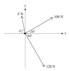
A small box of mass 40 kg is moved along a rough horizontal floor by three men. Two of the men apply horizontal forces of magnitudes 100 N and 120 N, making angles of 30° and 60° respectively with the positive x-direction. The third man applies a horizontal force of magnitude F N making an angle of  $\alpha$ ° with the negative x-direction (see diagram). The resultant of the three horizontal forces acting on the box is in the positive x-direction and has magnitude 136 N.
