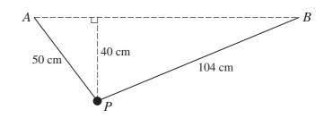
A particle P of mass 2.1 kg is attached to one end of each of two light inextensible strings. The other ends of the strings are attached to points A and B which are at the same horizontal level. P hangs in equilibrium at a point 40 cm below the level of A and B, and the strings PA and PB have lengths 50 cm and 104 cm respectively (see diagram). Show that the tension in the string PA is 20 N, and find the tension in the string PB. [5]
