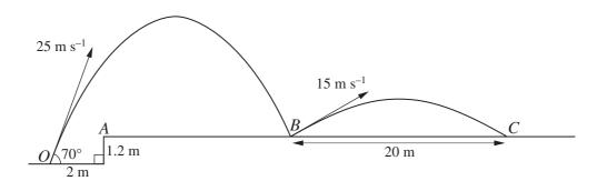
The point O is 1.2 m below rough horizontal ground ABC. A ball is projected from O with speed  $25 \,\mathrm{m\,s^{-1}}$  at an angle of  $70^\circ$  to the horizontal. The ball passes over the point A after travelling a horizontal distance of 2 m. The ball subsequently bounces once on the ground at B. The ball leaves B with speed  $15 \,\mathrm{m\,s^{-1}}$  and travels a further horizontal distance of 20 m before landing at C (see diagram).
