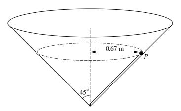
A particle P is moving inside a smooth hollow cone which has its vertex downwards and its axis vertical, and whose semi-vertical angle is  $45^{\circ}$ . A light inextensible string parallel to the surface of the cone connects P to the vertex. P moves with constant angular speed in a horizontal circle of radius 0.67 m (see diagram). The tension in the string is equal to the weight of P. Calculate the angular speed of P. [6]
