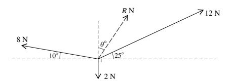
Three coplanar forces of magnitudes 8 N, 12 N and 2 N act at a point. The resultant of the forces has magnitude R N. The directions of the three forces and the resultant are shown in the diagram. Find R and  $\theta$ . [7]
