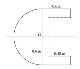
A cylindrical hole, of length 0.48 m, starting at the plane face of the solid, is made along the axis of symmetry (see diagram). The resulting solid has its centre of mass at *O*. Show that the area of the cross-section of the hole is  $\frac{3}{16}\pi$  m<sup>2</sup>. [4]
