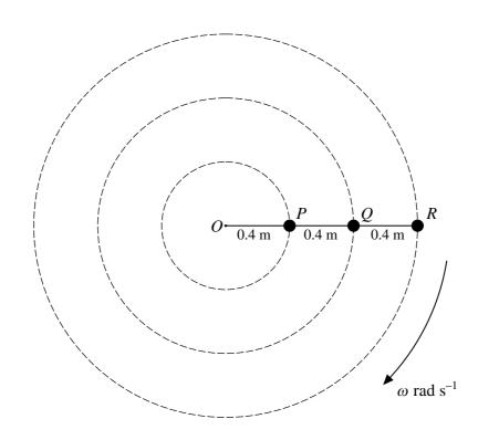
One end of a light inextensible string of length 1.2 m is attached to a fixed point O on a smooth horizontal surface. Particles P, Q and R are attached to the string so that OP = PQ = QR = 0.4 m. The particles rotate in horizontal circles about O with constant angular speed  $\omega$  rad s<sup>-1</sup> and with O, P, Q and R in a straight line (see diagram). R has mass 0.2 kg, and the tensions in the parts of the string attached to Q are 6 N and 10 N.
