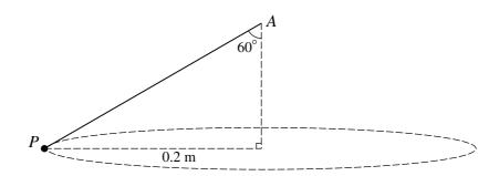
A particle P of mass  $0.4 \,\mathrm{kg}$  is attached to a fixed point A by a light inextensible string. The string is inclined at  $60^{\circ}$  to the vertical. P moves with constant speed in a horizontal circle of radius  $0.2 \,\mathrm{m}$ . The centre of the circle is vertically below A (see diagram).
