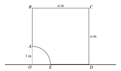
ABCDE is the cross-section through the centre of mass of a uniform prism resting in equilibrium with DE on a horizontal surface. The cross-section has the shape of a square OBCD with sides of length a m, from which a quadrant OAE of a circle of radius 1 m has been removed (see diagram).
