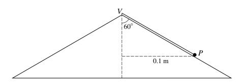
A particle *P* of mass 0.5 kg is attached to the vertex *V* of a fixed solid cone by a light inextensible string. *P* lies on the smooth curved surface of the cone and moves in a horizontal circle of radius 0.1 m with centre on the axis of the cone. The cone has semi-vertical angle  $60^{\circ}$  (see diagram).
