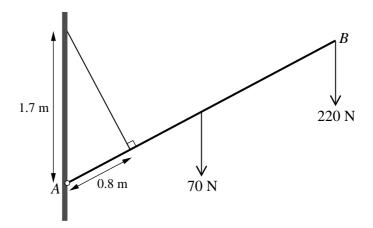
A uniform beam AB has length 2 m and weight 70 N. The beam is hinged at A to a fixed point on a vertical wall, and is held in equilibrium by a light inextensible rope. One end of the rope is attached to the wall at a point 1.7 m vertically above the hinge. The other end of the rope is attached to the beam at a point 0.8 m from A. The rope is at right angles to AB. The beam carries a load of weight 220 N at B (see diagram).
