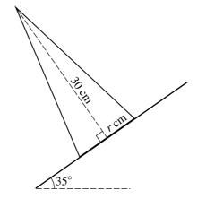
A uniform solid cone has height 30 cm and base radius r cm. The cone is placed with its axis vertical on a rough horizontal plane. The plane is slowly tilted and the cone remains in equilibrium until the angle of inclination of the plane reaches  $35^{\circ}$ , when the cone topples. The diagram shows a cross-section of the cone.
