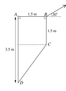
A uniform lamina of weight 15 N is in the form of a trapezium ABCD with dimensions as shown in the diagram. The lamina is freely hinged at A to a fixed point. One end of a light inextensible string is attached to the lamina at B. The lamina is in equilibrium with AB horizontal; the string is taut and in the same vertical plane as the lamina, and makes an angle of 30° upwards from the horizontal (see diagram). Find the tension in the string. [5]
