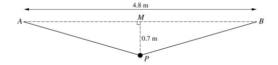
A particle P of mass 0.35 kg is attached to the mid-point of a light elastic string of natural length 4 m. The ends of the string are attached to fixed points A and B which are 4.8 m apart at the same horizontal level. P hangs in equilibrium at a point 0.7 m vertically below the mid-point M of AB (see diagram).
