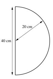
A frame consists of a uniform semicircular wire of radius 20 cm and mass 2 kg, and a uniform straight wire of length 40 cm and mass 0.9 kg. The ends of the semicircular wire are attached to the ends of the straight wire (see diagram). Find the distance of the centre of mass of the frame from the straight wire. [4]
