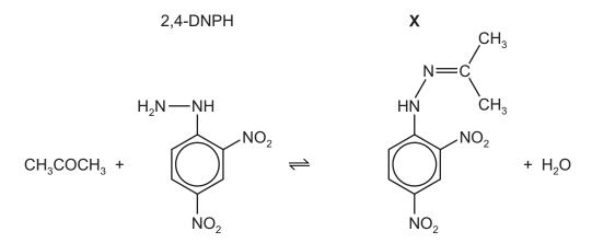
The melting point of **X** can be used to confirm the identity of the carbonyl compound that has reacted with 2,4-DNPH. To do this, solid **X** must be separated from the mixture.
