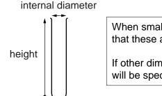
When small test-tubes are provided, it is expected that these are approximately 150 mm in height.
