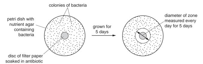
The table shows the results of testing five different types of bacteria. Zones of less than 13 mm show the presence of resistant bacteria.
