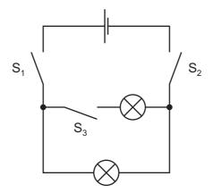
Which switches must be closed so that both lamps light?
