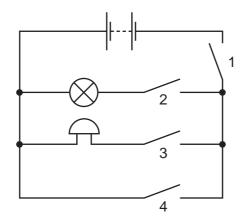
Which switches must be closed for the bell to ring without lighting the lamp?
