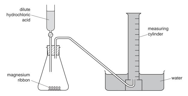
30 cm<sup>3</sup> of dilute hydrochloric acid were added to the conical flask containing magnesium ribbon. The timer was then started and the volume of gas collected in the measuring cylinder was measured every 20 seconds for 180 seconds (3 minutes).
